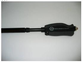
Step 3: Adjust the clutch as follows: To Loosen: Turn the hexagon nut to the left. To Tighten: Turn the hexagon nut to the right.
