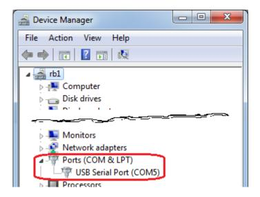
• In the resulting list, look for the number of the COM port that your computer has assigned to the VGM-1041's USB Serial Port (in the case shown it's COM 5).
