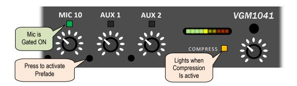
If you play the audio source you have connected to the AUX inputs earlier, you'll hear both the mic and the audio together (it's a mixer, after all!), from both your amplifier and the front-panel headphone jack.
